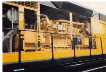
RL-2000 with access doors open
