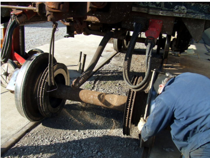
A wheelset is rolled out from under 1 of TCRM's passenger cars. Photo by Terry Bebout
